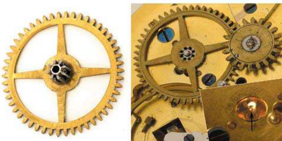
Picture 10: Wheel with pinion inside the train frame
