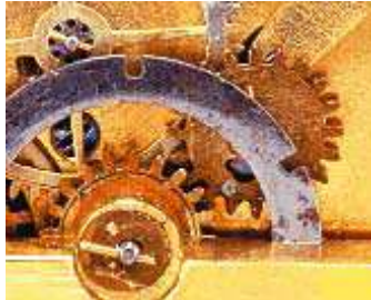
Picture 11: Details of the automatic winding gears
